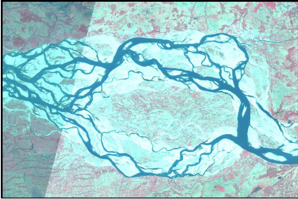
Fig. 12: The Moderately Braided Channels (Reach 3 - Palashbari Gumi) in IRS 1C LISS - III image of 1997 year with Plan Form Index value 2.4
