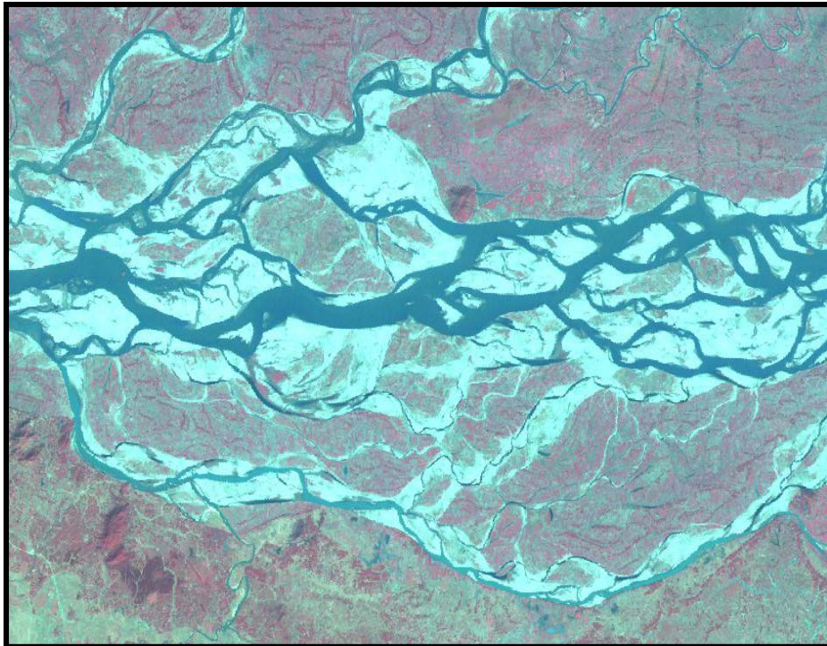
Fig. 10: The Moderately Braided Channels (Reach 2 – Near Barpeta) in IRS 1C LISS - III image of 1997 year with Plan Form Index value 4.1
